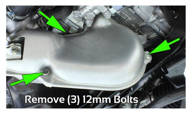
4. Remove (4) 12mm bolts securing right side, lower exhaust manifold heat shield to manifold. **NOTE: This** will not fall from car as 02 sensor will be holding it in place.
