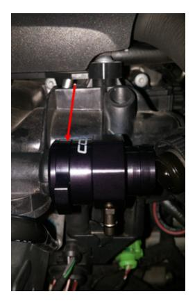
6. To finish the install, clip the hose onto the boost tap. This should clip right onto the barbed fitting of the boost tap just like it did stock.
