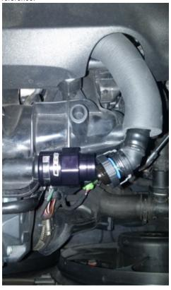
5. Take the retaining clip provided and clip the boost tap to the intake manifold. The clip slides over the grooves seen on the boost tap and will click into place.
