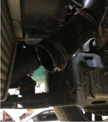
15. Now, we'll want to loosen and remove the entire driver side charge pipe. Do so by using a 7mm socket and loosen and remove all clamps. Pull the piping connecting the intercooler to the throttlebody out and set it all aside. We don't need it anymore.
