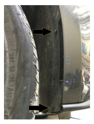
8. Once the fender rivets are removed, you'll be able to pull back the plastic liner to access the single 7mm bolt that is located up at the corner of each side of the bumper. This bolt holds the corners of the bumper to the front quarter panels. This needs to be removed completely on both sides before attempting to remove the bumper.
