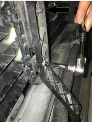
12. With the grille shutters out, we need to remove this cross bar at the front of the frame rails. Use a 10mm socket to remove the four (4) bolts and set the cross bar aside.
