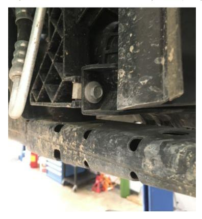
18. Now, on the driver side, there is clip system that you must unclip. From here, you should be able to start getting the intercooler removed. You may need to push back on the radiator, twist in all sorts of strange ways, but eventually, you'll get this FMIC out. Just take care not to damage any fins on the radiator or intercooler in the process. Just be patient, you'll get it!
