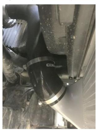
6. At this point, your intercooler is fully installed, just loosely. Now is when you need to take some time to make some adjustments to how the piping is fitting onto the intercooler, where the brackets are located, etc. The intercooler fits the best when it is positioned as far back
