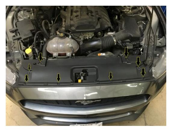
4. Using an 8mm socket, remove the six (6) screws that line the top of the bumper, as seen with the vertical arrows below.
