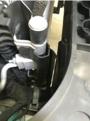
14. With the panels removed, now it's time to finally remove the factory FMIC. Using a 7mm socket and extension, loosen the bottom most hose clamp that connects the passenger side charge pipe to the intercooler and pull it away from the intercooler. Bend it up and out of the way.
