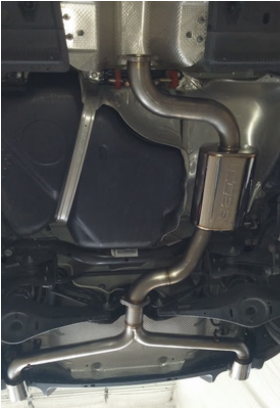
8. Place one gasket with two 10mm flange bolts on the open end of the downpipe.
