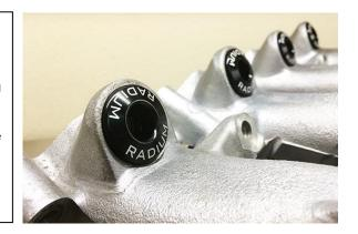
6. Position the fuel rail in place making sure all injectors are lined up properly in the Radium injector seats. Next, press firmly on the fuel rail to seat the injectors' lower O-rings.
