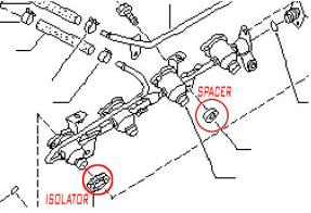
3. The 20-0558 fuel rail was designed around specific a fuel injector height and O-ring dimensions. Reference the fuel rail product page or contact <a href="mailto:info@radiumauto.com">info@radiumauto.com</a> for more information.
