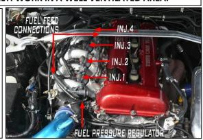
2. Use a 12mm socket wrench to remove the M8 fuel rail mounting bolts.
