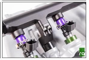
8. Using the OEM fuel rail spacers, position the fuel rail assembly onto the intake manifold. Install the OEM M8 bolts and torque to 15ftlbs (21Nm) using a 12mm socket wrench.
