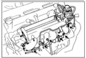
4. After the engine has cooled, place shop towels down under the fuel inlet pipe. Slowly loosen the banjo bolt and catch any gasoline that drips out.
