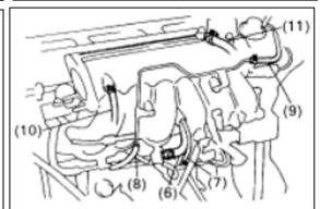
3. Disconnect EGR gas temperature sensor connector.
