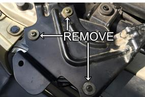
3. Remove the 3 OEM rubber mounting grommets from the OEM bracket, as shown. Be careful not to damage these, as they will be reused.
