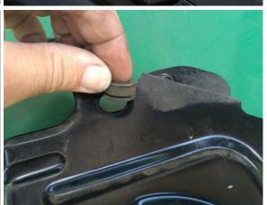
4. Install the rubber grommets into the Radium bracket. Mount the cruise control module using the OEM plastic-tapping screws.
