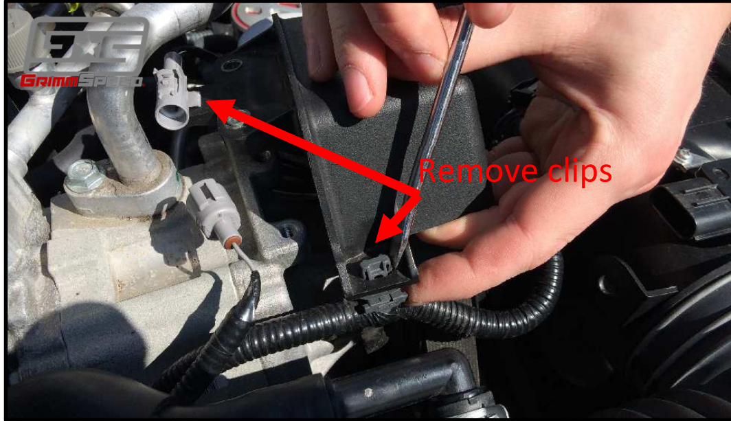
Figure 4: Remove wiring harness clips from oem cover
