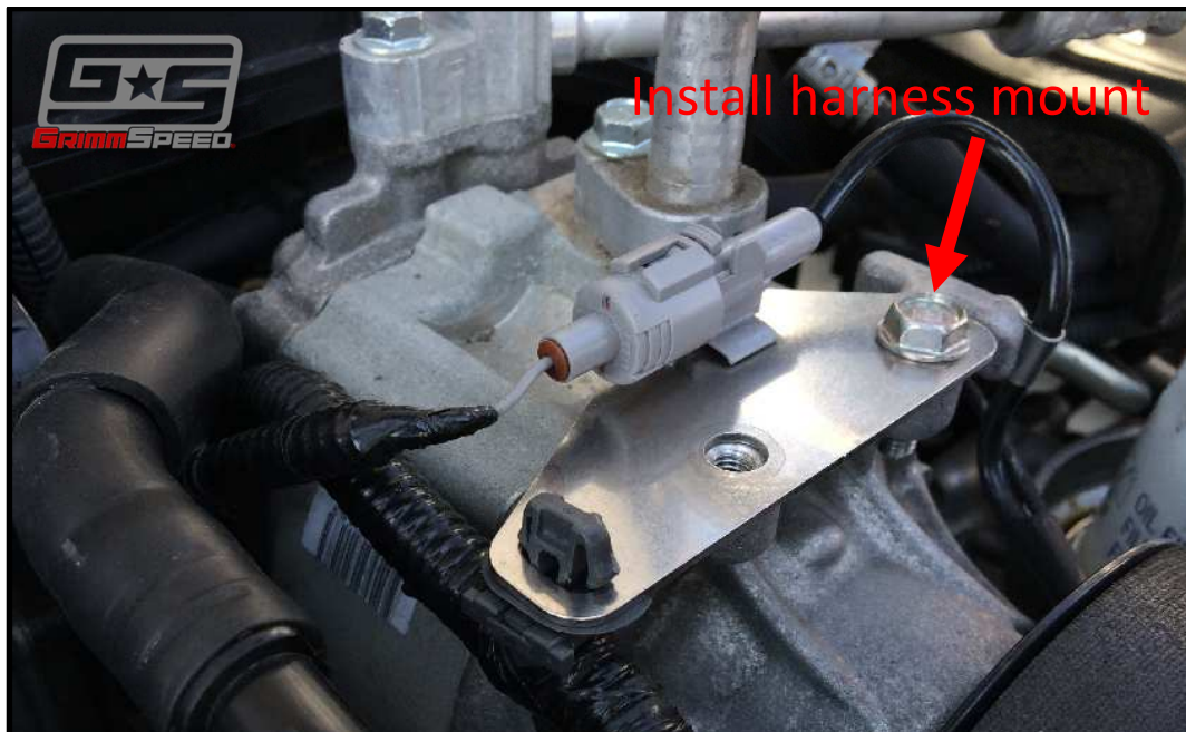
Figure 5: Install GrimmSpeed harness mount
