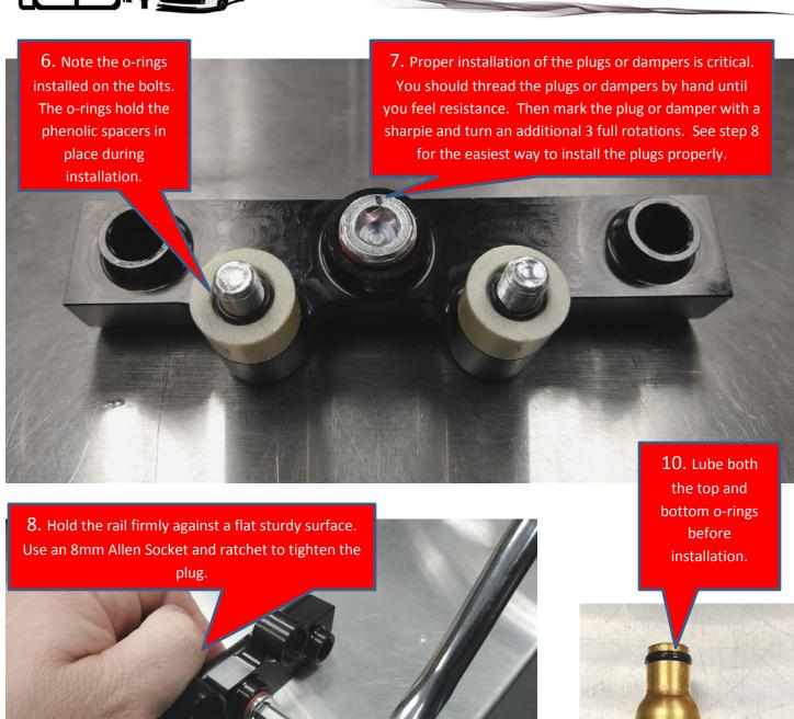
PRO TIP — Install masking tape on the back of the fuel rail to prevent scratching during this step.
