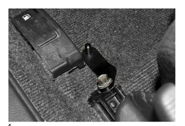
5. Place the floor mat back in the vehicle and slide the hole over the stud as shown.
