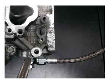
4. Install a 12mm banjo fitting on the AVCS port and point the male fitting away from the cylinder head. Run the braided line that comes out of the side of the tee fitting to the banjo fitting. Tighten the line with a  $^9/_{16}$ " wrench. Torque the banjo bolt to 24  $^{\rm ft}/_{\rm lbs}$ .
