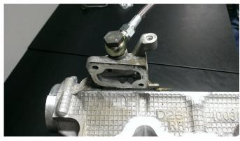
10. Install the 90° -4 AN fitting onto the oil restrictor on the top of the turbo. Tighten the line with a  $^9/_{16}$ " wrench.
