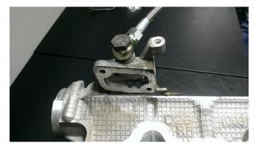
6. Install the 90° -4 AN fitting onto the oil restrictor on the top of the turbo. Tighten the line with a  $\frac{9}{16}$ " wrench.
