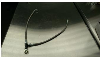
8. Using the banjo bolt that came out of the back of the head, assemble the tee fitting on the back oil port of the head as shown. Use a thinner washer between the head of the banjo bolt and the banjo. Then use the thicker washer between the banjo and the engine. This is the only place to use a thick washer.
