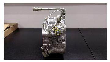
2. Install the supplied oil plug in the top oil port. Use a 12mm crush washer between the head and plug. Torque the plug to 24  $^{\rm ft}/_{\rm ls}$ .
