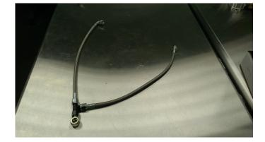
3. Using the banjo bolt that came out of the back of the head, assemble the tee fitting on the back oil port of the head as shown. Use a thinner washer between the head of the banjo bolt and the banjo. Then use the thicker washer between the banjo and the engine. This is the only place to use a thick washer.
