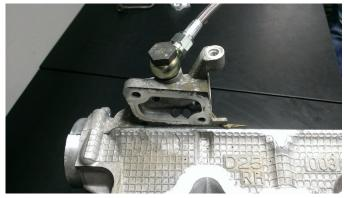
5. Install the 90° -4 AN fitting onto the oil restrictor on the top of the turbo. Tighten the line with a  $^9/_{16}$ " wrench.
