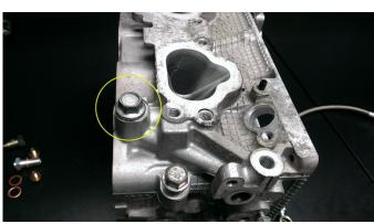
3. Assemble one 12mm banjo on the bottom port of the tee fitting. The braided line with the straight fittings is installed on the middle port and the braided line with the 90° fitting is installed on the top port as shown. The 90° fitting will be installed on the top of the turbo. It is important that the face of the banjo fitting be parallel with the side of the t-fitting. Tighten all 3 fittings with a  $^9/_{16}$ " wrench.
