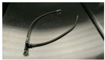
3. Using the banjo bolt that came out of the back of the head, assemble the tee fitting on the back oil port of the head as shown. Use a thinner washer between the head of the banjo bolt and the banjo. Then use the thicker washer between the banjo and the engine. This will be the only place to use a thick washer.
