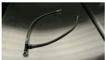
4. Using the banjo bolt that came out of the back of the head, assemble the tee fitting on the back oil port of the head as shown. Use a thinner washer between the head of the banjo bolt and the banjo. Then use the thicker washer between the banjo and the engine. This will be the only place to use a thick washer.
