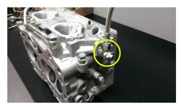
4. Run the other end of the braided line to the turbo oil feed port and install the 10mm banjo bolt. Tighten the line with a  $^9/_{16}$ " wrench. Torque the banjo bolt to 16  $^{\rm ft}/_{\rm lbs}$ .
