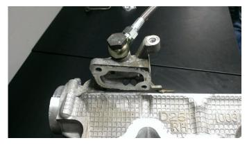
6. Install the 10mm banjo fitting on the top of turbo using the existing banjo bolt. Put a 10mm copper washer on each side of the banjo fitting.
