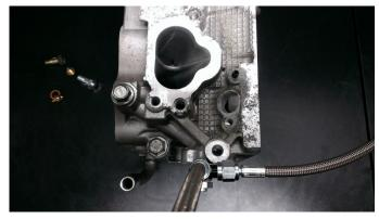
5. Install a 12mm banjo fitting on the AVCS port and point the male fitting away from the cylinder head. Run the braided line that comes out of the side of the tee fitting to the banjo fitting. Tighten the line with a  $^9/_{16}$ " wrench. Torque the banjo bolt to 24  $^{\rm ft}/_{\rm lbs}$ .
