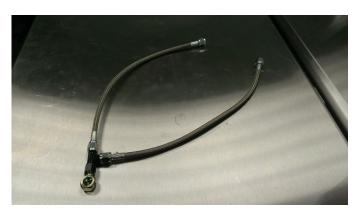
8. Using the banjo bolt that came out of the back of the head, assemble the tee fitting on the back oil port of the head as shown. Use a thinner washer between the head of the banjo bolt and the banjo. Then use the thicker washer between the banjo and the engine. This is the only place to use a thick washer.
