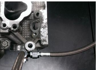
4. Install a 12mm banjo fitting on the AVCS port and point the male fitting away from the cylinder head. Run the braided line that comes out of the side of the tee fitting to the banjo fitting. Tighten the line with a  $^9/_{16}$ " wrench. Torque the banjo bolt to 24  $^{\rm ft}/_{\rm lbs}$ .
