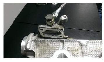
10. Install the 10mm banjo fitting on the top of turbo using the existing banjo bolt. Put a 10mm copper washer on each side of the banjo fitting.
