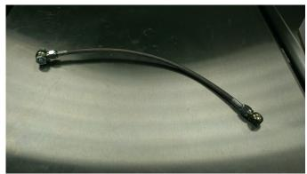
3. Using the banjo bolt that came out of the back of the head, assemble the banjo on the back oil port of the head as shown. Use a thinner washer between the head of the banjo bolt and the banjo. Then use the thicker washer between the banjo and the engine. This is the only place to use a thick washer. Torque the banjo bolt to 24 ft/lbs.
