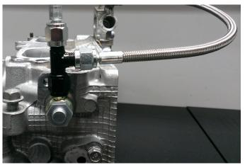
9. Install a 12mm banjo fitting on the AVCS port and point the male fitting away from the cylinder head. Run the braided line that comes out of the side of the tee fitting to the banjo fitting. Tighten the line with a  $^9/_{16}$ " wrench. Torque the banjo bolt to 24  $^{\rm ft}/_{\rm lbs}$ .
