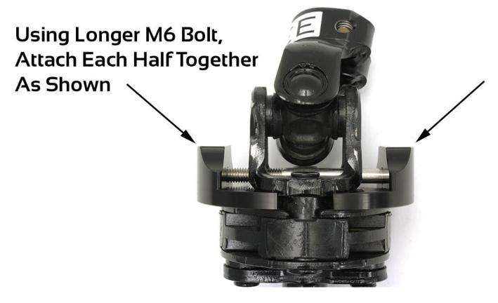
5. Using supplied wrench, slowly tighten bolt compressing both halves together. Once the bolt is tight (both halves should be touching upper half of universal joint and bolt will be sticking out of one side) remove bolt from PERRIN Steering Dampener Lockdown.
