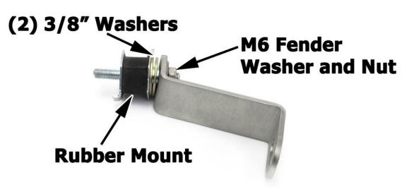
9. Install supplied bracket (with rubber mount) to threaded hole in frame rail and secure using supplied M6 screw and fender washer. Leave loose until air intake pipe is mounted.
