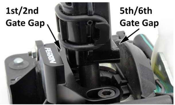
Above picture shows shifter in neutral. Actual gaps when  $\mathbf{1}^{st}/2^{nd}$  gear or  $\mathbf{5}^{th}/6^{th}$  gear are selected, will be much smaller.
