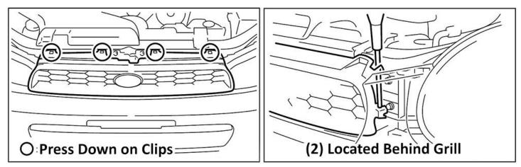
b. For 06-07 cars, on center grill, remove (2) small plastic fasteners from top section. Carefully pull grill straight out from bumper to expose mounting location. There are 4 large clips holding this in place and they can be kind of tight while removing.
