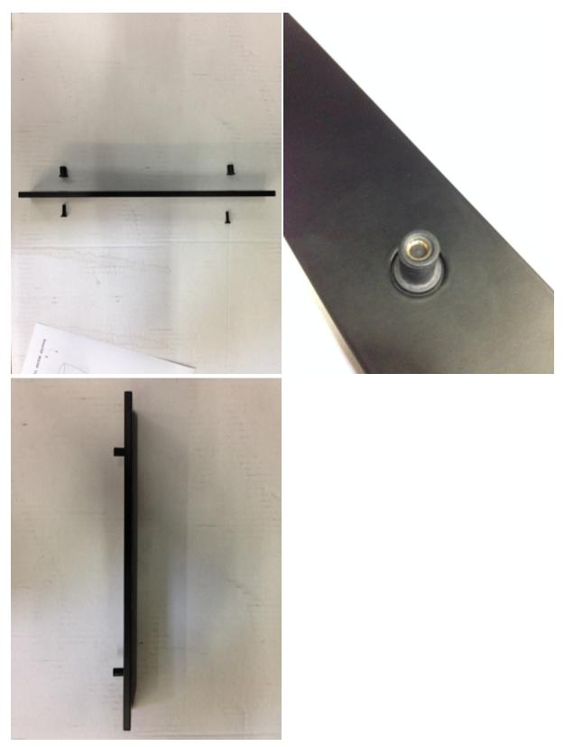
3. With the license plate delete now assembled it is time to install it onto the car. With the "COBB" logo facing the correct way, insert the rubber rivet nuts into the stock holes on the front bumper.
