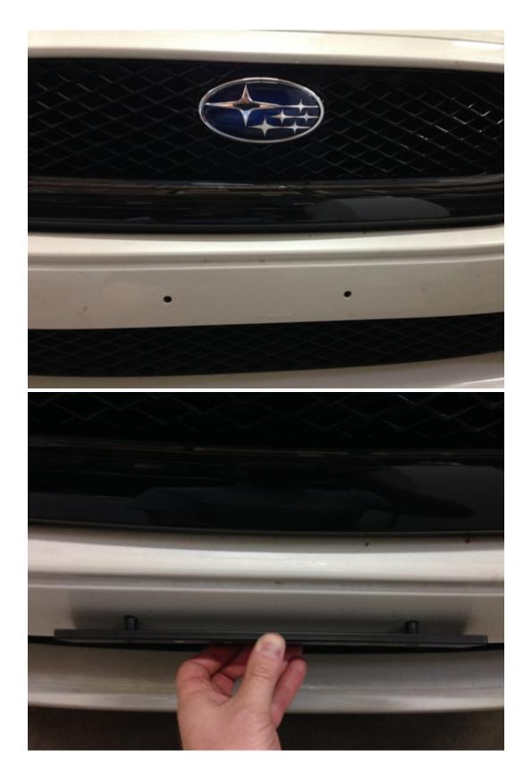
4. Once the license plate delete is in place on the car, you can begin to tighten the rubber rivet nuts so that the rubber expands and secures the plate to the car. When doing this be sure that the plate delete remains flush against the car. Once both of the rivet nuts are tightened, be sure to give the plate delete a tug to ensure that it was installed properly. Enjoy your new COBB Front License Plate Delete!
