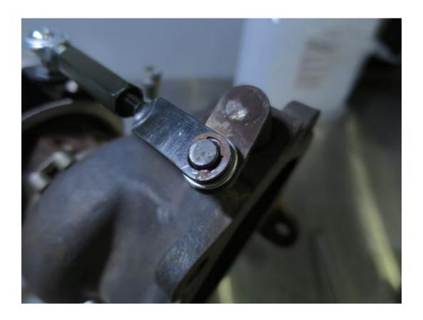
5. Using a M12 socket or wrench, tighten up the bracket bolts.
