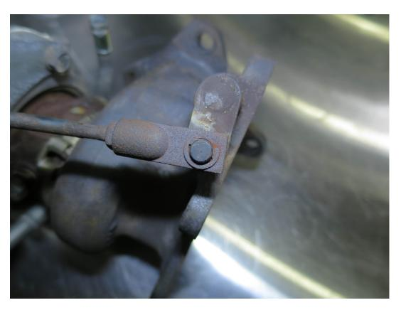
3. Using a small flat blade screwdriver pop the clip out of place, making sure not to lose it as you'll need it later on. (An easy way to keep it with you is to put your hand over the assembly so that it pops into your and as it comes off. If your screwdriver fits in the gap between the pin and the clip, you can simply rotate it around and it should pop the clip out.
