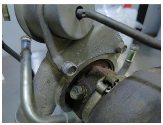
2. With the bolts cracked loose but not removed, turn your attention to the wastegate actuator arm, and locate the E-Clip holding it in place
