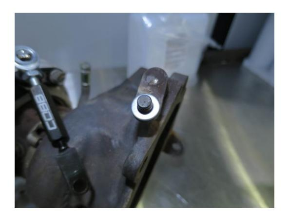
3. With that in place go ahead and install the ball socket end of the IWG arm onto the bracket, making sure to use a washer underneath. Then tighten using 2 11mm wrenches.
