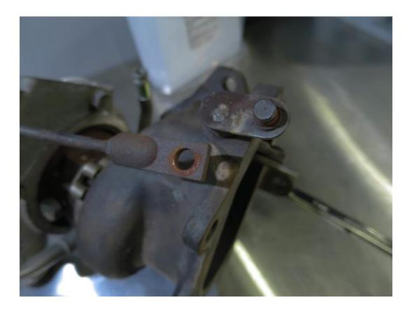
5. Now you can go ahead and remove the entire actuator assembly from the turbo.
