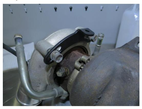
2. Now go ahead and place the M6 washer onto the pivot pin on the wastegate actuator arm. If your turbo has a hole instead, you will use the provided bolt, nut, and washer.
