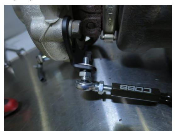
4. Now go ahead and slip the other end over the wastegate actuator pin and push on the old e-clip. You may need to loosen this up by spinning the center collar of the arm to adjust the length.
