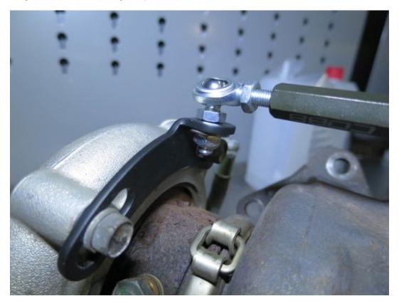
6. Spin the center section of the arm to go ahead and adjust the wastegate all the way closed. Or all the way open if you're trying to make the car really boring to drive.
