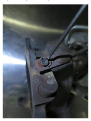
4. Once the clip is removed, go ahead and pull the actuator arm free, be careful as it will likely be under spring loaded tension from the actuator and can come off with a bit of force.
