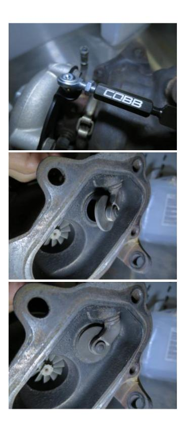
7. Once you're done go ahead and spin the jam nut down towards the center collar, then tighten it by turning the jam nut towards the collar, and the collar towards the jam nut using two 11mm wrenches.
