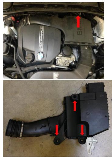
6. Unscrew the T30 Torx screw that holds the charge pipe to the motor
