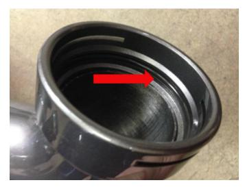
3. Install the silicone reducer onto the charge pipe with the 048 hose clamp, and tighten using an 8mm socket.
