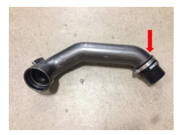
4. Install the COBB Charge Pipe on the car first making sure the throttle body section is seated properly. The throttle body side is typically going to be the most common place to see leaks from improper installation so make sure it is all the way in place and seated properly before moving on. Once seated install the stock c-clip in the same orientation used on the stock charge pipe.
