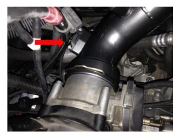
6. Slide the silicone reducer over the aftermarket or stock intercooler pipe and tighten the 040 hose clamp using an 8mm socket or nut driver.
