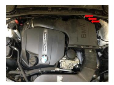
3. Detach the air scoop from the airbox by disengaging the nub from the plastic retainer (1 on each side)
