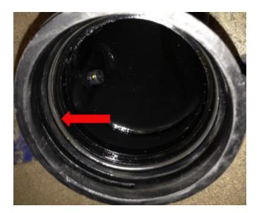
11. Using a T20 Torx bit, remove the MAP sensor from the stock charge pipe. It will be reused on the COBB Charge Pipe so set it somewhere safe and take care not to damage the sensor end.
