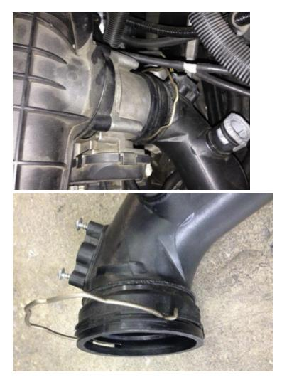
9. Disconnect the wire harness from the MAP sensor on the back of the charge pipe. It may be easier to pull the charge pipe off of the throttle body and intercooler pipe in order to get to the clip.
