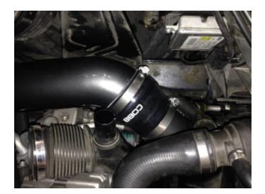
7. Reinstall the factory intake by reconnecting and fastening the inlet tube and pressing down on the airbox to seat the 3 rubber retainers.
