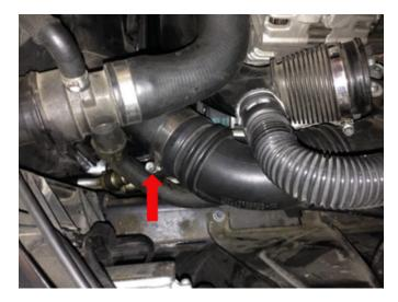
8. Remove the c-clip that holds the charge pipe to the throttle body with a screwdriver. Take great care not to lose it as BMW doesn't like selling these individually and they are difficult or expensive to otherwise source.
