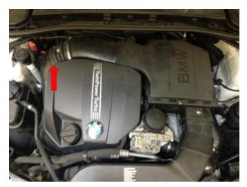
2. Remove the 3 rubber wire holders from the rear of the airbox.
