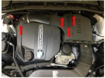
8. Reattach the 3 rubber cable holders to the airbox.
