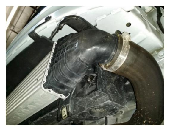
3. Next utilize a 7mm socket to loosen the hose clamp that attaches the factory piping to the turbo at theback of the motor. Also, use a 13mm socket to remove the two (2) 13mm nuts that hold the pipe to the bottom of the motor. Remove the pipe.
