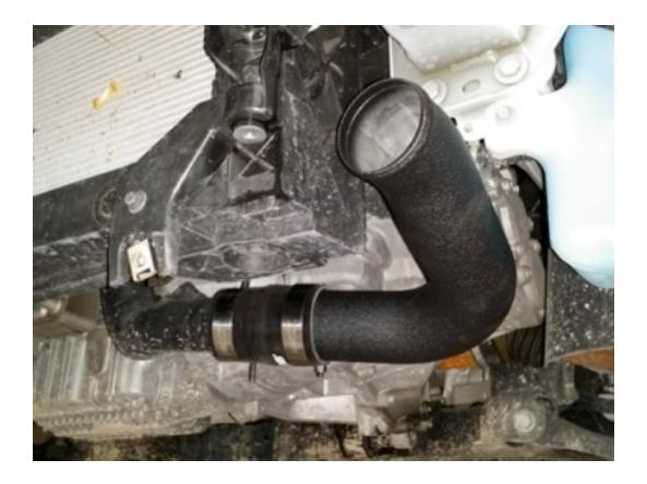
2. Use the smaller T-bolt clamp to install the 2.5" to 1.5 " reducer onto the turbo outlet and tighten it down.
