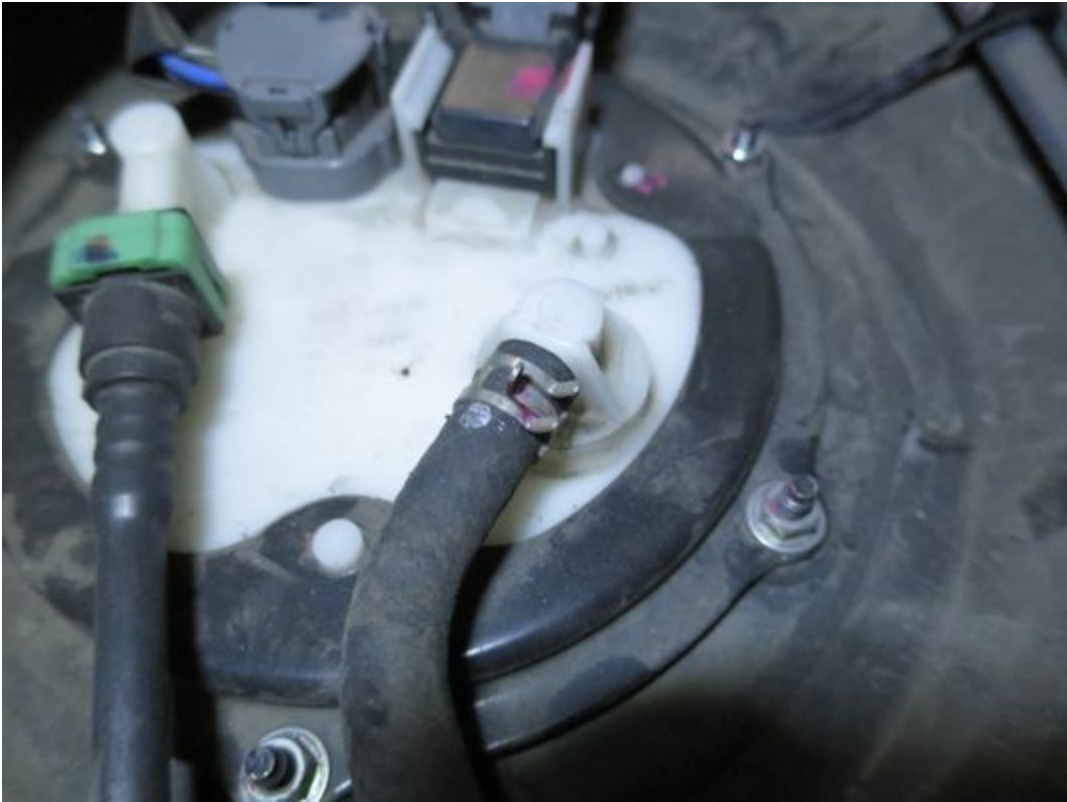
9. Now undo the flip on the other fuel line and pull that fuel line free.
