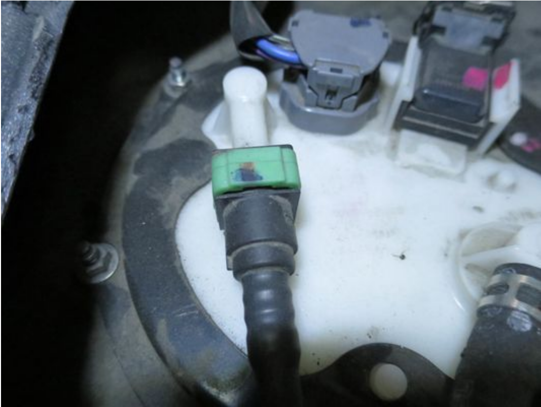
9. Now undo the flip on the other fuel line and pull that fuel line free.
