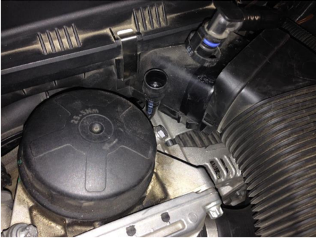
7. Detach the scoop from the airbox by pulling the plastic over the retaining clips (one on each side) and remove the air scoop.
