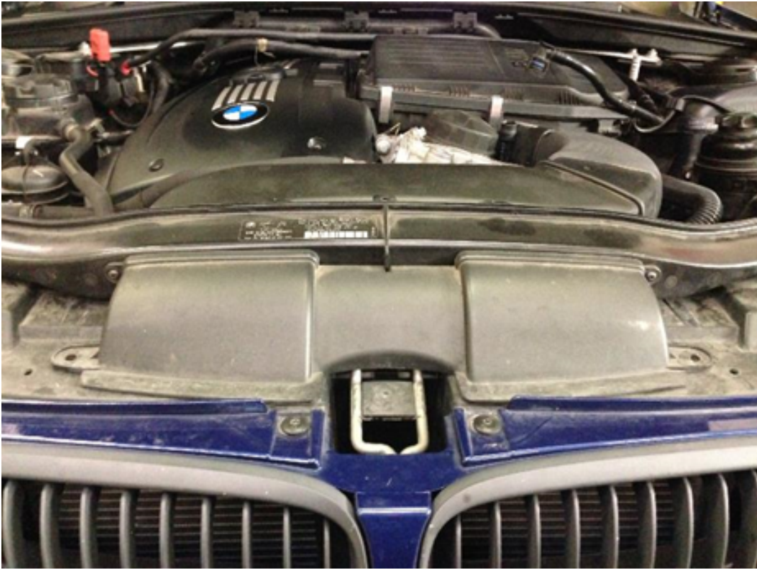
7. Detach the scoop from the airbox by pulling the plastic over the retaining clips (one on each side) and remove the air scoop.
