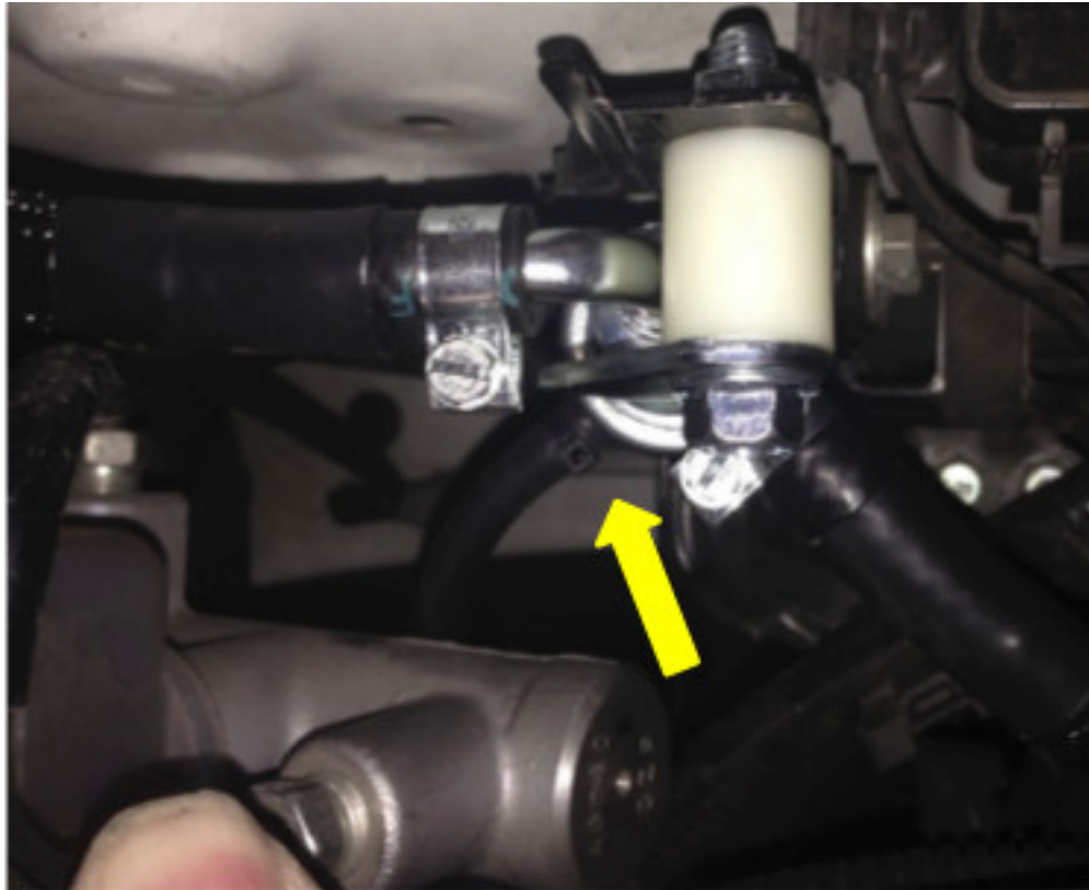
9. Feed Line Orientation – Install the feed line with the sheath covered section going towards the fuel rails.
