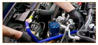
13. Slip a hose clamp over the other end of this hose and install it to the port marked IN on the catch can. (1x worm-gear clamp)
