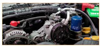
**08.** Remove the pop-clips that secure the crankcase vent hose to the intake manifold. (2x pop-clips)
