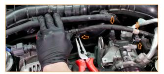
07. Remove the four bolts that secure the AC compressor and engine hook. Then remove the engine hook and move the compressor forward to expose the CCV port underneath. [4x 14mm bolts]
