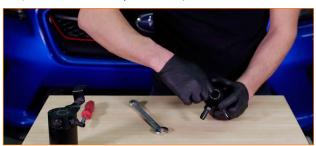
02. Remove the two pop-clips that secure the intake air duct to the radiator support. Then remove the intake air duct. (2x pop-clips)
