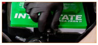
12. Locate the hose with three bends in your kit. Lead the end with the 90° bend under the electrical harness and AC lines as shown here. Slip a worm-gear clamp over the end of the hose and install it to the CCV port on the engine. Now tighten the clamp to secure the hose. (1x worm-gear clamp)
