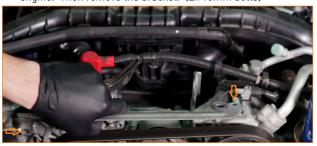
05. Take note of how the belt is routed and draw a diagram for later. Then take the tension off the belt and remove it from the AC compressor pulley. The tensioner bolt is a 14mm fastener.
