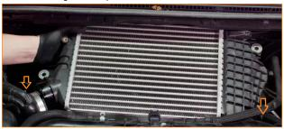
25. Remove the bolts that secure the driver-side intercooler mounting bracket. Then remove the bracket. Note that the longer bolt is the one that secures the intercooler to the bracket. (3x 12mm bolts)
