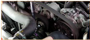
06. Release the harness clips that secure the alternator cable and disconnect the electrical harness from the AC compressor. Then lift the alternator cable out of the harness clips and tuck it back. Disconnect the alternator cable from the intake manifold by compressing the tabs on the clip and sliding it out of the manifold.
