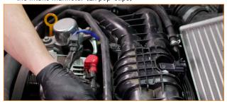
09. Reach down behind the AC compressor and compress the clamp that secures the CCV hose to the engine. Then separate the hose from the engine. (1x spring-clamp)
