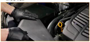
03. Remove the two pop-clips that secure the back of the plastic engine cover. Then remove the engine cover from the vehicle by lifting it from the front edge. The front edge is held on with two pegs and grommets. (2x pop-clips)
