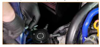
30. Locate the hose with the single 90° bend. Note that one end of this hose has a larger diameter outlet. Slip a worm-gear clamp over the end with the 90° bend, then install this to the port marked OUT on the catch can. Lead the wide end of the hose under the wiring harness. Lead it underneath the hoses at the back of the manifold and install a worm-gear clamp over the end. (1x worm-gear clamp)
