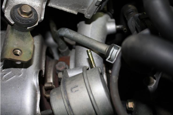
5. And remove the hose from the pressure side of the turbo.
