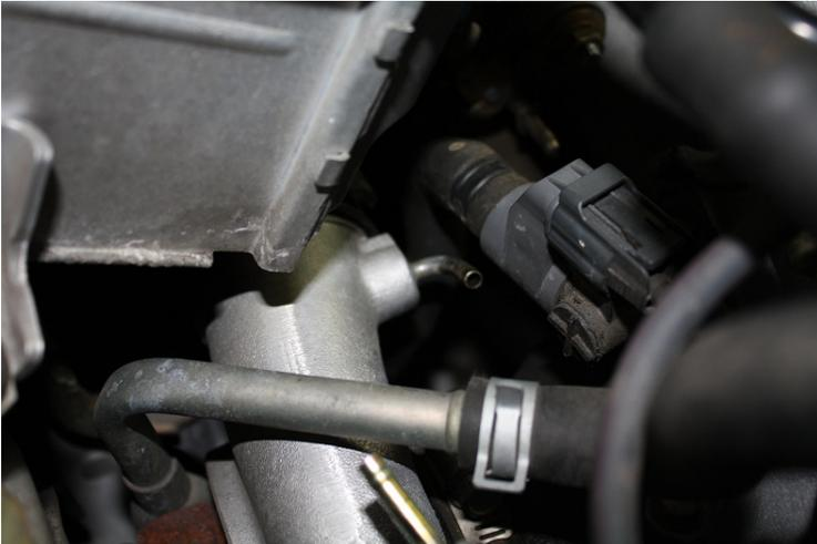
6. Connect the pressure source (compressor side of turbo, intake manifold, etc) to the inlet on the GrimmSpeed manual boost controller using the supplied vacuum line. The inlet side is at the bottom of the manual boost controller. See Fig. A. Tighten hose ends with zip ties.
