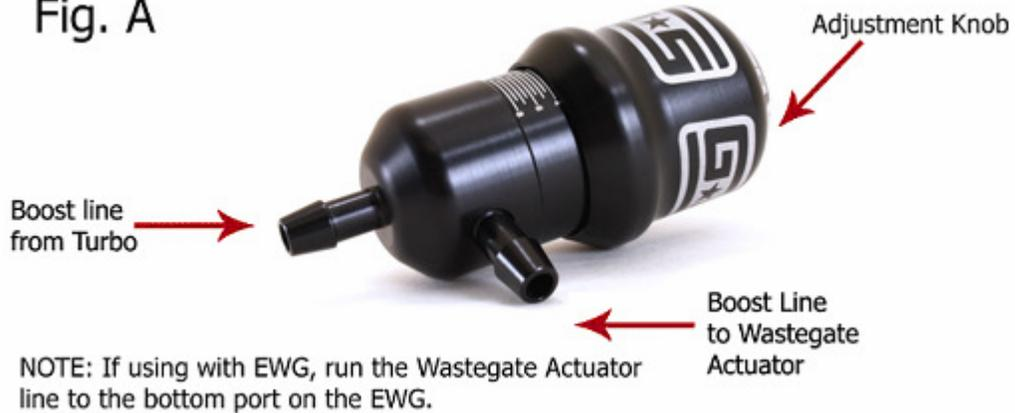
10. Turn adjustment knob CLOCKWISE to INCREASE boost pressure. Turn adjustment knob COUNTER-CLOCKWISE to DECREASE boost pressure (see end of adjuster for correct rotation direction). We advise starting at a lower boost pressure and then working your way up to your desired target boost pressure. Each click equals approximately one quarter of a psi. Each rotation equals one line on the scale and there are 16 clicks per rotation.
