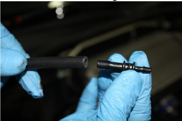
8. Connect the wastegate actuator to the outlet of the manual boost controller with the supplied vacuum line. The outlet side of the manual boost controller is on the side of the boost controller. See Fig. A. Tighten hose ends with supplied zip ties.
