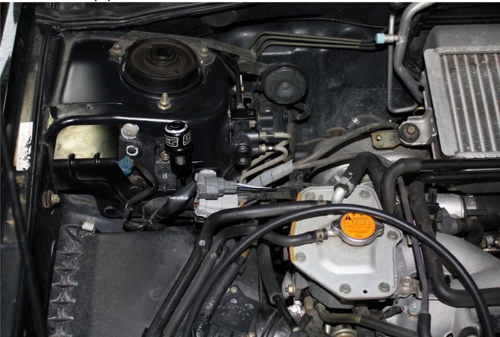
3. You will now remove all OEM boost controlling vacuum lines. (This includes removing any restrictive pills). If the vehicle uses a boost control solenoid, we recommend leaving the electrical connector plugged in to avoid check engine lights but you will still remove the vacuum lines that are connected to it.
