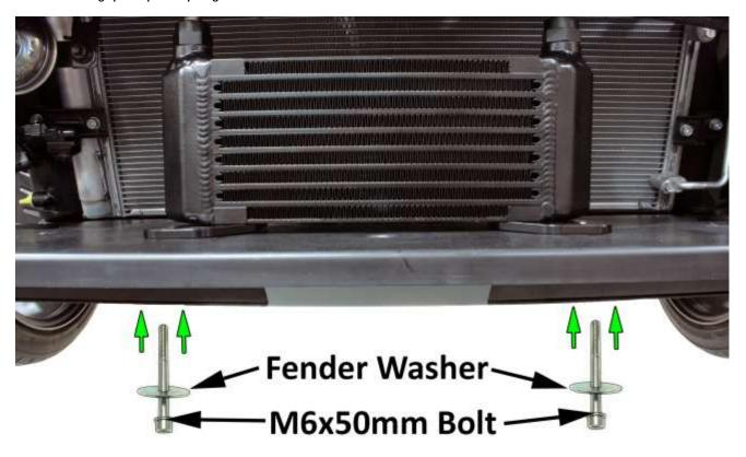
17. Go back through all fittings and adjust the angles and then tighten them down. This step may require readjusting of hoses and fittings to ensure hoses line up and clear things properly. NOTE: The oil hoses will touch on certain parts of the car and this is perfectly ok. The PERRIN
