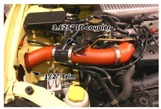
17. Inside fender well, locate intake pipe and bracket. These should be resting on top of one another. Place filter onto pipe keeping in mind that the hose clamp will go around bracket and filter at the same time. Loosen clamp around filter enough to get bracket under clamp.
