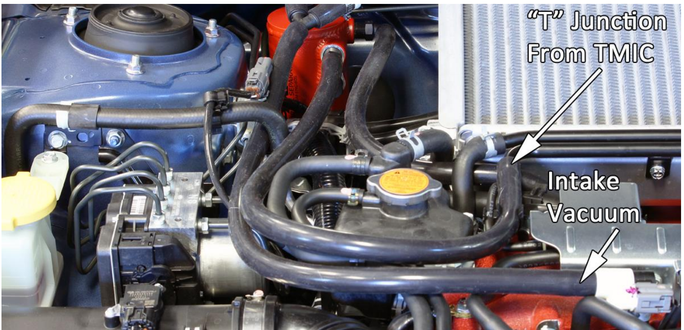
Above picture shows intake vacuum source at turbo inlet hose on 2012+ STI engine with extra PCV diagnosis connector.
