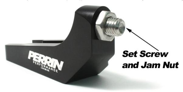
7. Using (1) supplied M6x20 bolt in hole closest to M12 Set screw, Install PERRIN Master Cylinder Support to chassis as shown below. NOTE: Align with (2) M6 threaded holes in shock tower, not holes without threads.
