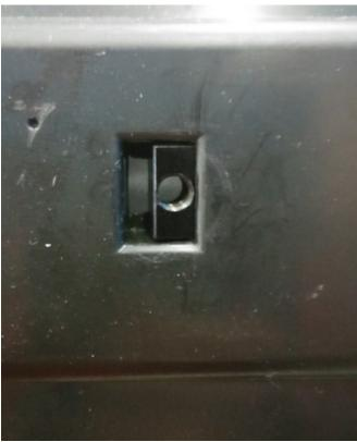
2. Insert one of the provided screws through one of the holes on the license plate delete. Line this screw up with the corresponding anchor in the bumper cover and begin to tighten, leaving some slack. Repeat this process for the opposite side.
