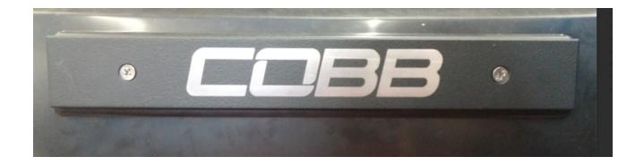
3. Tighten both screws until the license plate delete is tightly secured.
