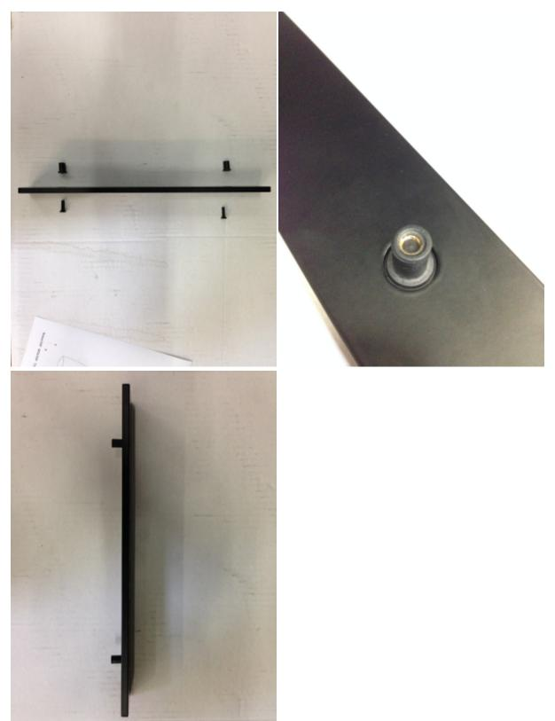
3. With the license plate delete now assembled it is time to install it onto the car. With the "COBB" logo facing the correct way, insert the rubber rivet nuts into the stock holes on the front bumper.
