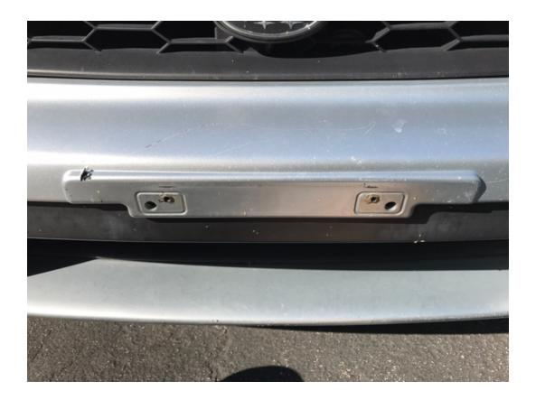
4. Once the license plate delete is in place on the car, you can begin to tighten the rubber rivet nuts so that the rubber expands and secures the plate to the car. When doing this be sure that the plate delete remains flush against the car. Once both of the rivet nuts are tightened, be sure to give the plate delete a tug to ensure that it was installed properly. Enjoy your new COBB Front License Plate Delete!
