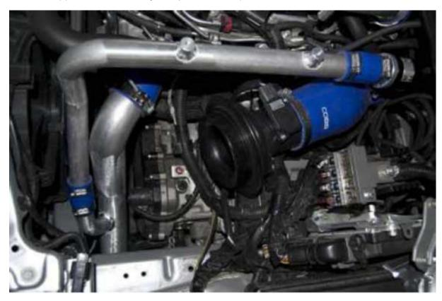
2. Install the upper intercooler pipe by first removing the two rubber grommets from the factory intercooler pipe. Push out the metal sleeve and then the grommet. Reinstall the rubber grommets and sleeves into the COBB intercooler pipe bracket.
