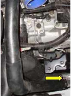
4. Remove the large plastic cover on top of the radiator support by removing the three plastic fasteners.
