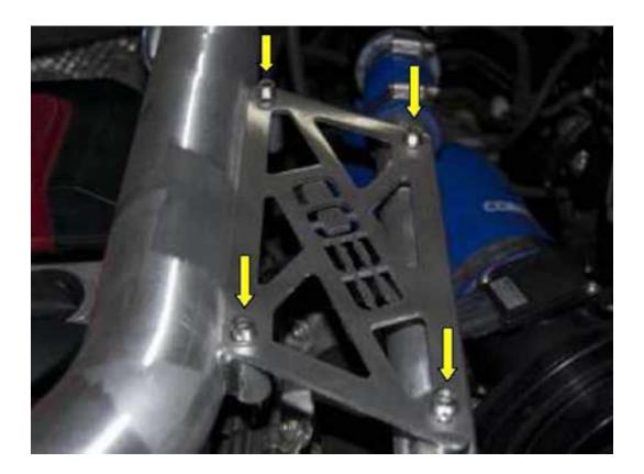
7. Temporarily install the air box and air intake duct. By adjusting the orientation of the pipes you should be able to get the BPV pipe to sit in the cutout in the intake duct. Some minor trimming may be required.
