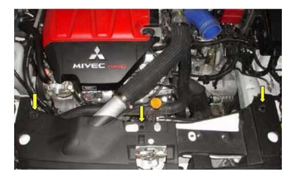
5. Remove the rear portion of the upper intercooler pipe by loosening the two 10mm hose clamps securing the upper intercooler pipe to the turbo inlet and the aluminum intercooler inlet tube.
