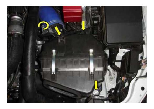
3. Loosen the two 10mm hose lamps that secure the long rubber BPV hose and remove it.
