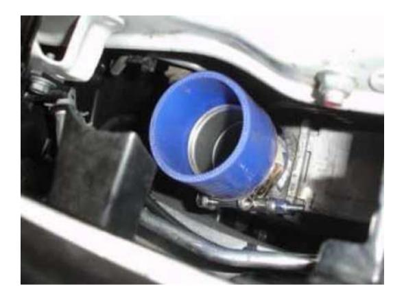
5. Slide the upper intercooler pipe into the silicone reducer on the turbo outlet first, and then onto the intercooler inlet. Before tightening any of the clamps you will want to first reinstall the two 12mm bolts into the bracket on top of the radiator core support.
