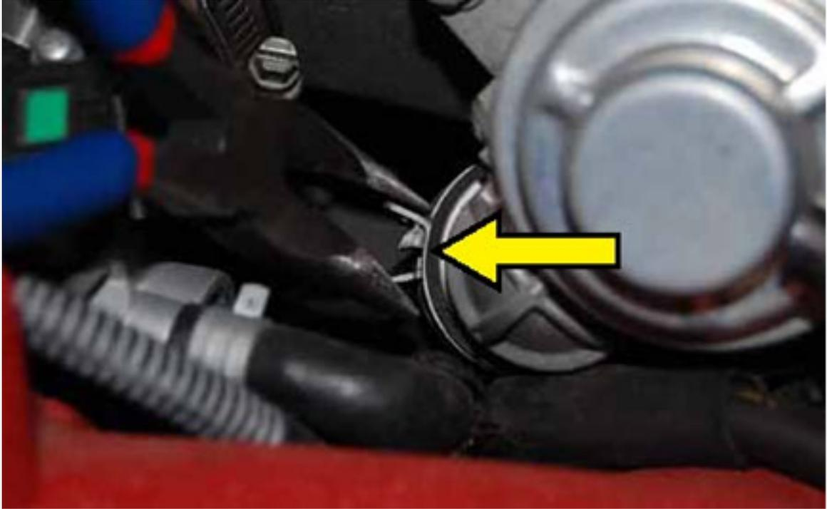
3. Remove the vacuum line from the factory bypass valve.
