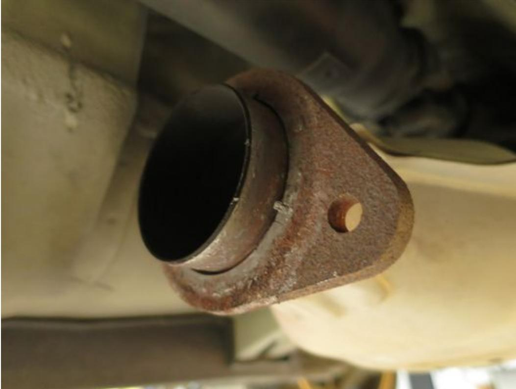
2. If damaged (like ours was) replace the gasket.
