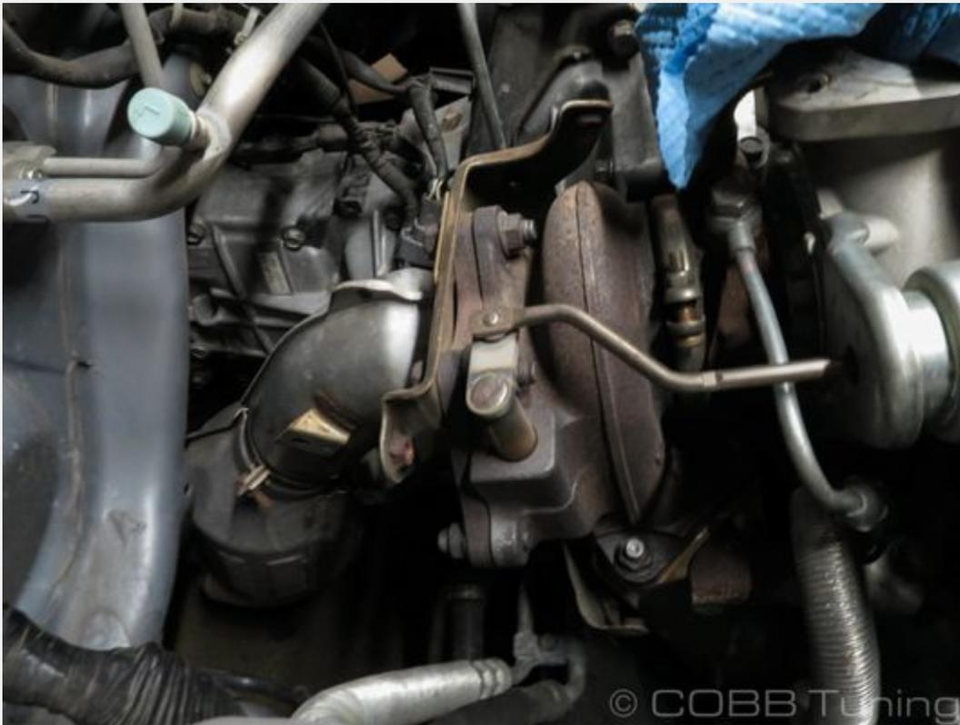
5. Now is a good time to check out the heat shield bracket as the factory units are quite prone to cracking and damage. Replace yours as needed.
