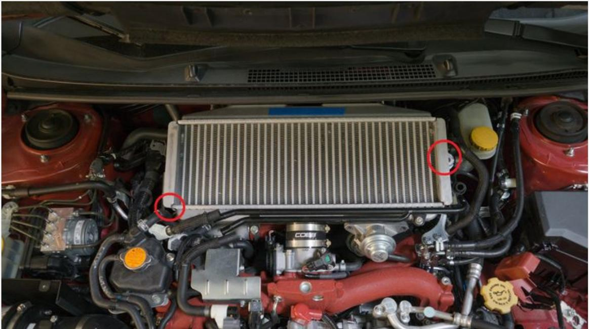
9. Gently wiggle TMIC free from engine bay by sliding it back and then out. Be careful to not damage your windshield wiper cowl.
