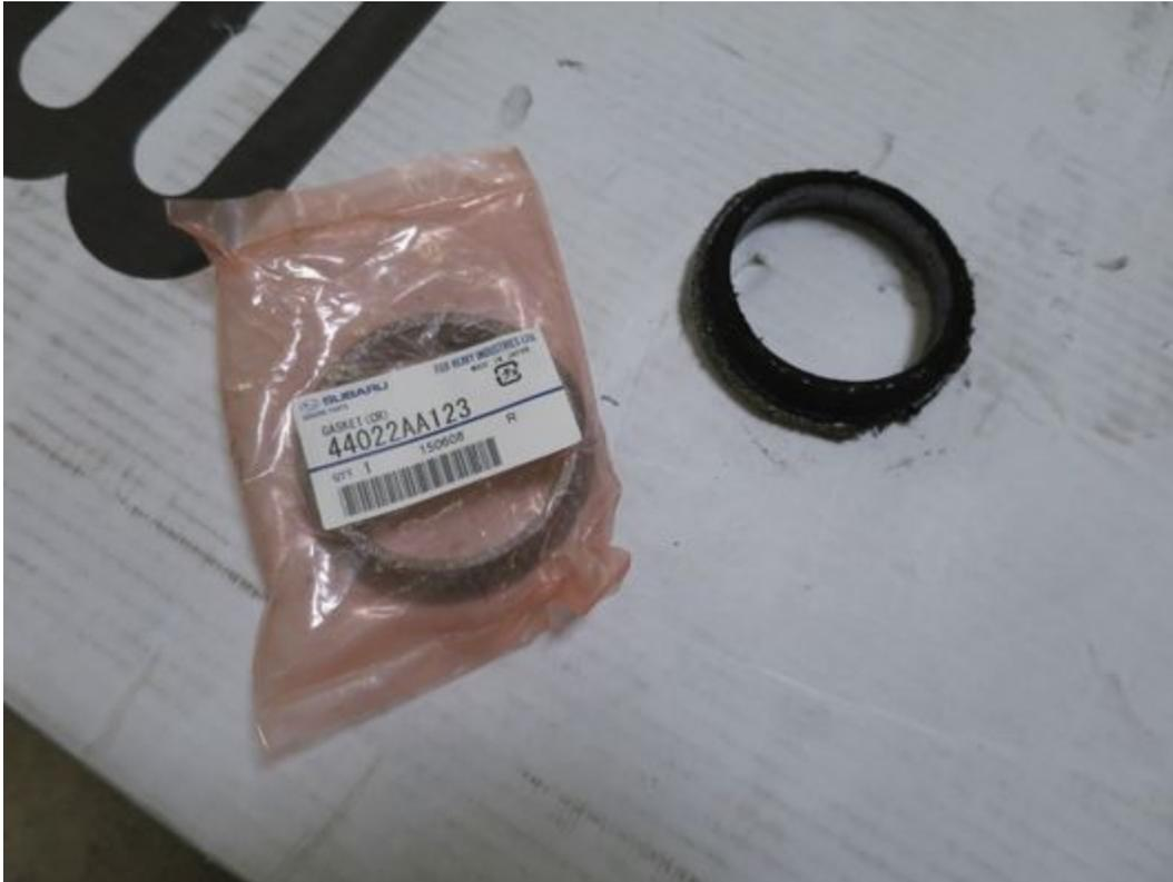
3. The new gasket should simply slide into place on the new downpipe.
