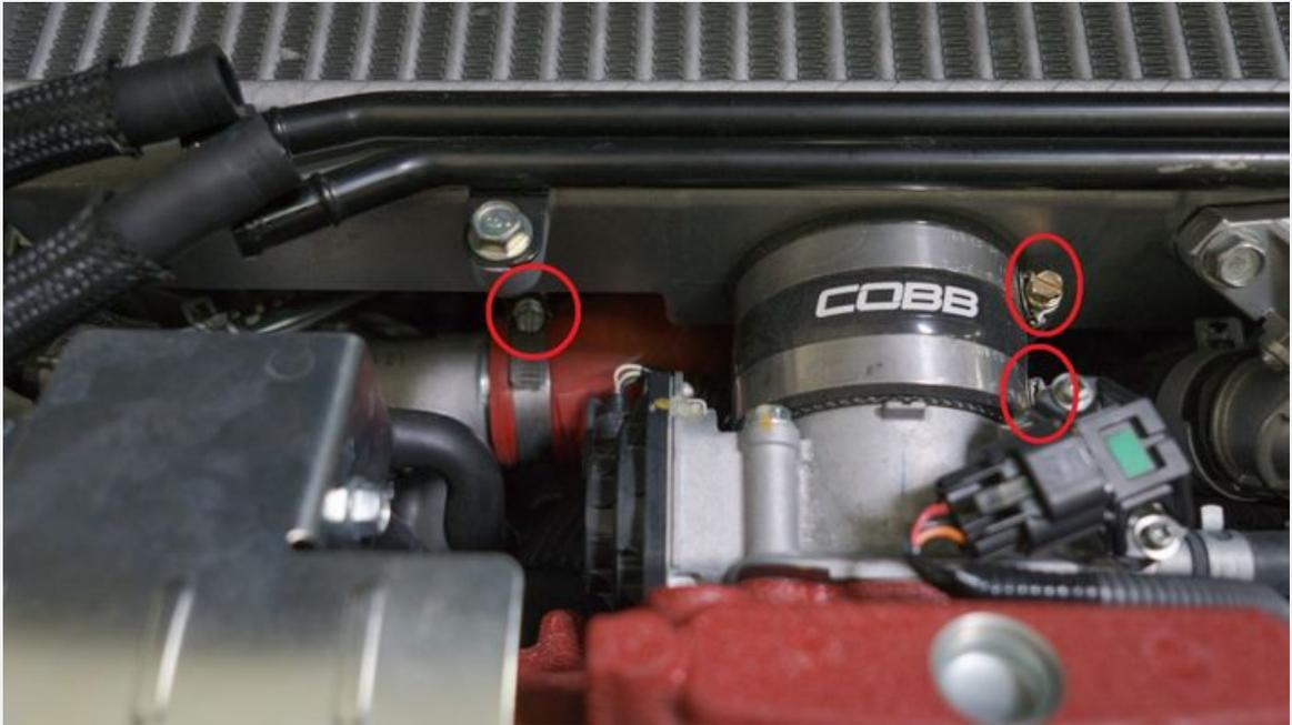
8. Remove the two bolts securing the intercooler to its brackets.
