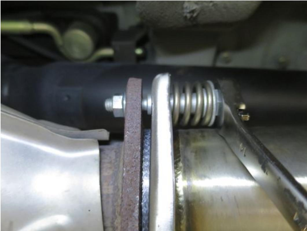
7. Using a 22mm oxygen sensor wrench or socket remove the stock O2 sensor (This may also be a good candidate for some penetrating oil).
