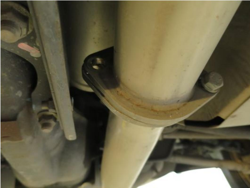
6. With the one bolt in the rear supporting the exhaust support the mid-pipe with your hand and undo the exhaust hanger. Hanger pliers make this job infinitely easier.
