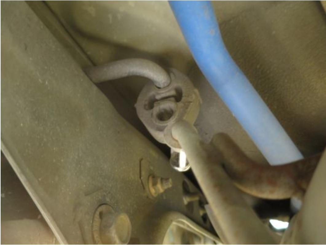
9. Now remove the hanger towards the inside of the car (USD M Passenger). If it doesn't come off easily you may need to remove the rear diffuser (if equipped). Make sure to support your exhaust at this point to ensure it doesn't drop.
