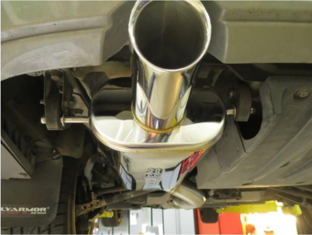
7. Once everything is in, use the provided hardware and gasket between the midpipe and muffler, and leave hand tight.
