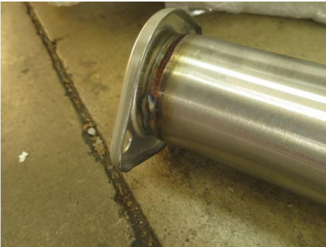
5. If noone ruined your downpipe flange previously, you should be able to reuse the OEM spring bolts and thread them into the downpipe and leave them loose. If someone ruined your flange previously, you'll need to add exhaust or locking nuts on the back side to get things
