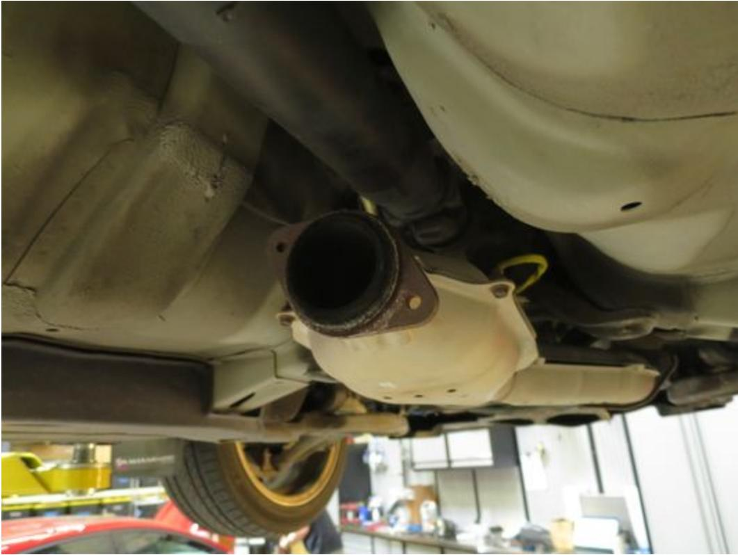
8. Middle section removed, we can turn our attention to the rear section. Start by removing the rear hanger close to the differential and swaybar.
