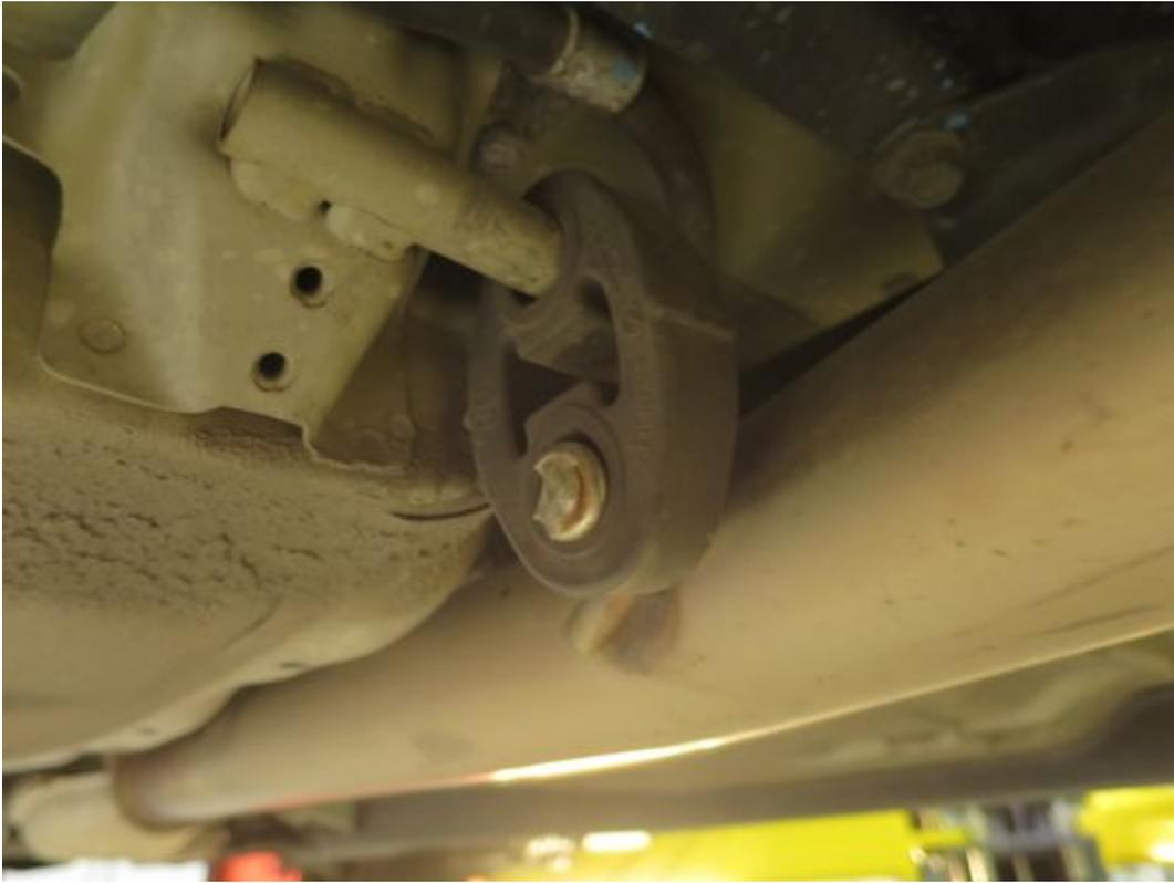
7. With the center hanger removed go ahead and pull the remaining bolt on the mid-pipe and remove it from the car.
