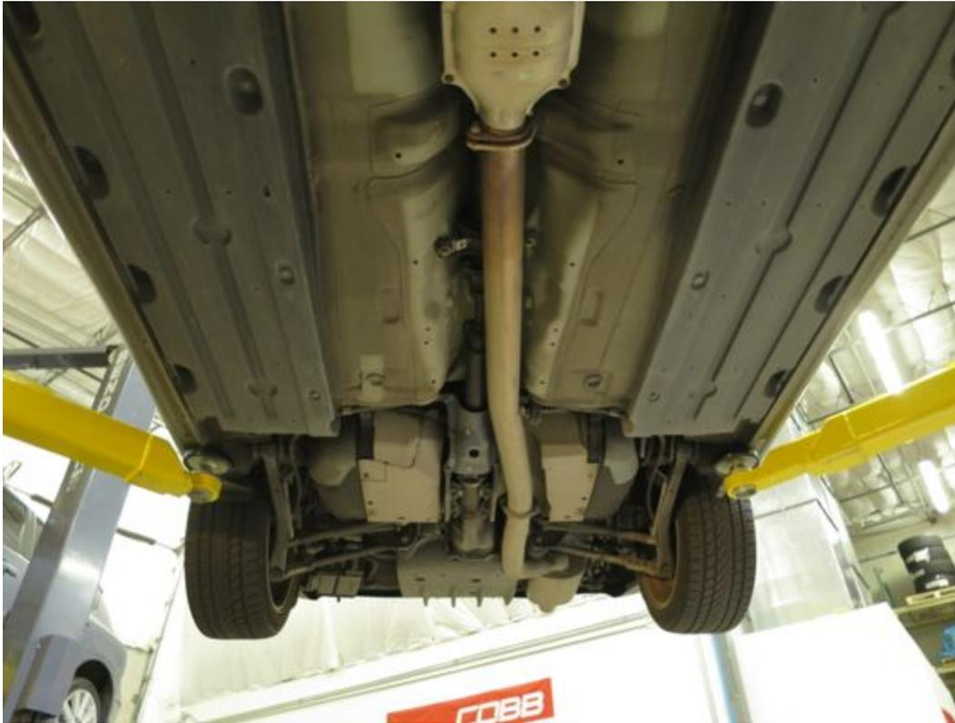
3. Go around and lubricate your exhaust hangers with silicon lube (one on the mid pipe and three on the rear muffler) and all the exhaust bolts with a penetrating oil to allow for easy removal.
