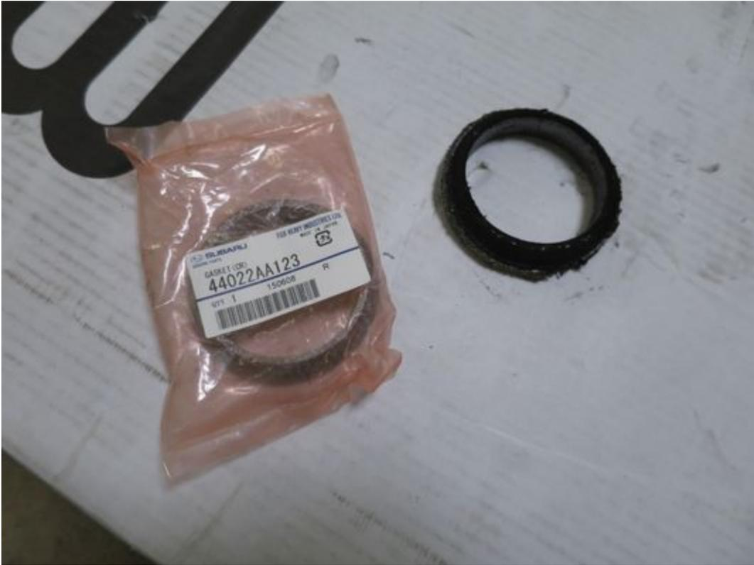
3. The new gasket should just slip in place on the downpipe.
