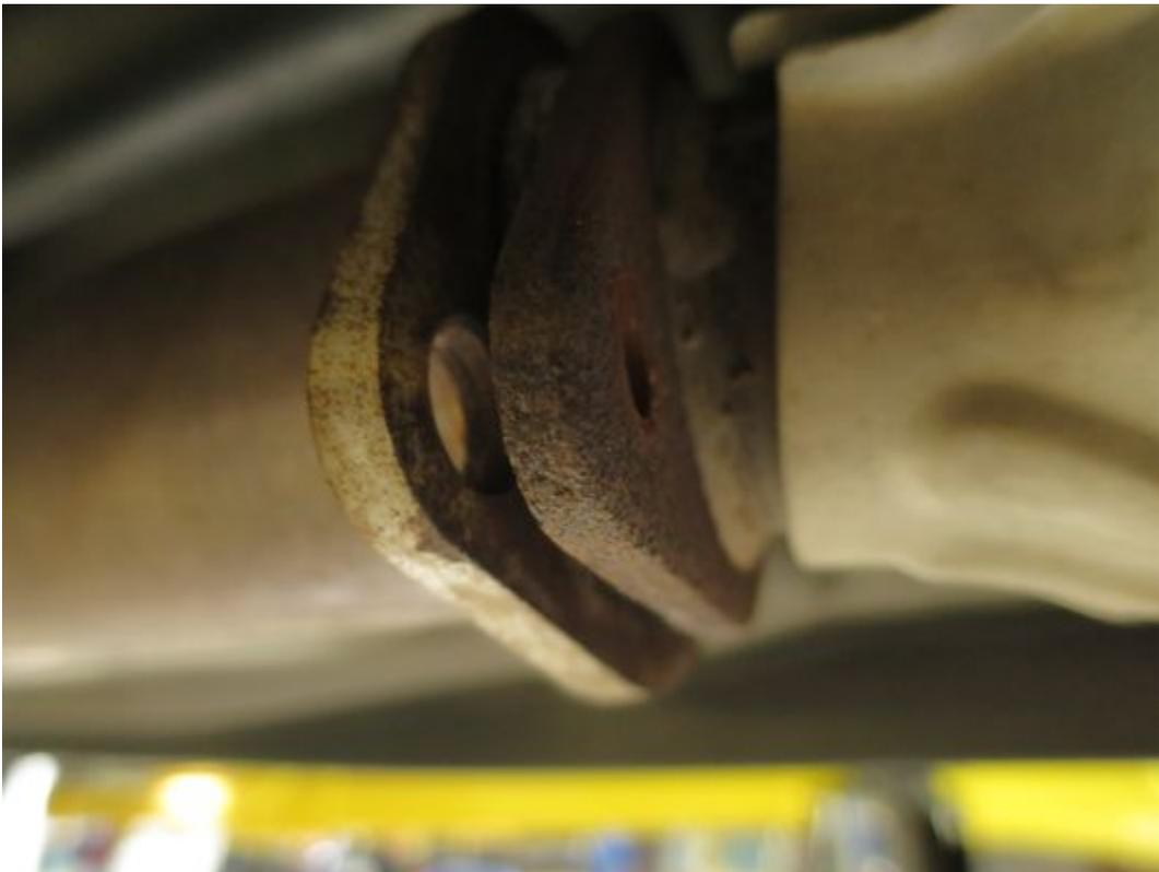
5. Using two 14mm wrenches or a 14mm wrench and socket take one of the rear bolts from the midpipe and leave the other one hand tight.
