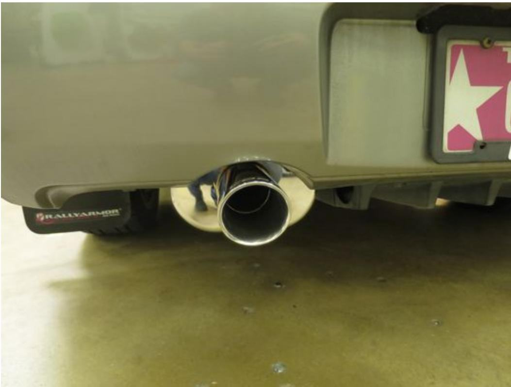
9. Once it's where you want it, tighten things down starting in the front. The spring bolts naturally bottom out at a certain point so don't over tighten them with your 14mm socket. And remember, this flange is designed to allow some movement.
