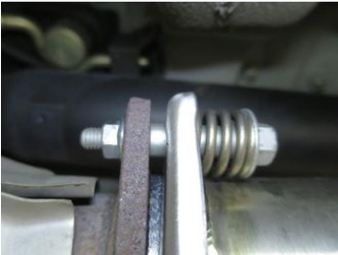
10. With that tightened, you'll want to tighten the rear flange. Keep in mind that due to differences in manufacturing (both the car and the exhaust) as well as the age of the vehicle, getting your muffler to look perfect will most likely not leave the flanges lined up perfectly, however the exhaust will seal regardless so you should be good to go.
