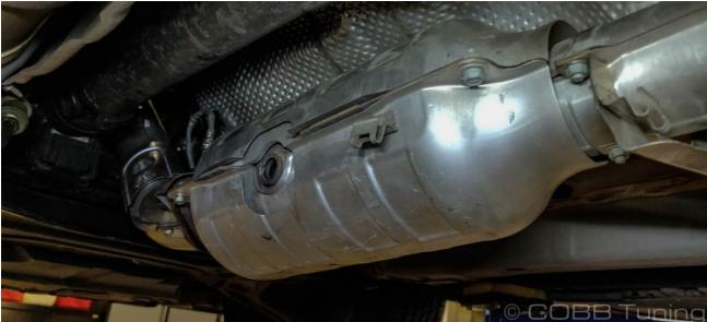
4. Unbolt the side exhaust hanger using a 12mm wrench.
