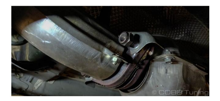
6. Loosen the two 19mm rear bolts of the mid-pipe. Once they're both moving easily you can remove both of the bolts entirely.
