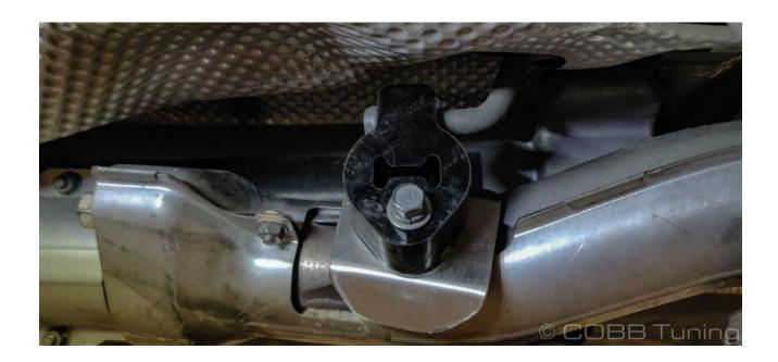
5. Loosen the two 19mm nuts going from the downpipe to the factory mid-pipe. Leave the nuts on loosely for now to give you the support to loosen the remaining bolts.
