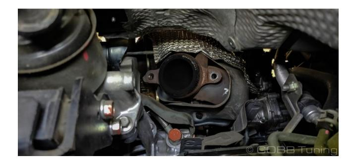
10. The stock donut gasket is reused so make sure yours is in good shape and replace as needed.
