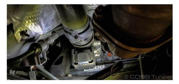
3. Use the provided gasket and hardware to bolt the rear of the downpipe to the midpipe (if using a COBB midpipe). If you're hooking it up to the factory catted mid-pipe you'll use the provided gasket and the factory hardware to bolt it on to the studs of the mid-pipe.
