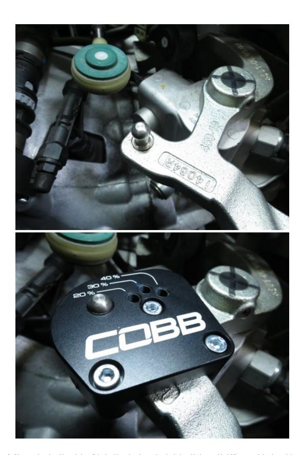
9. Now go ahead and loosely install the backing plate by turning the bolts with the provided Allen wrench but leave it loose.
