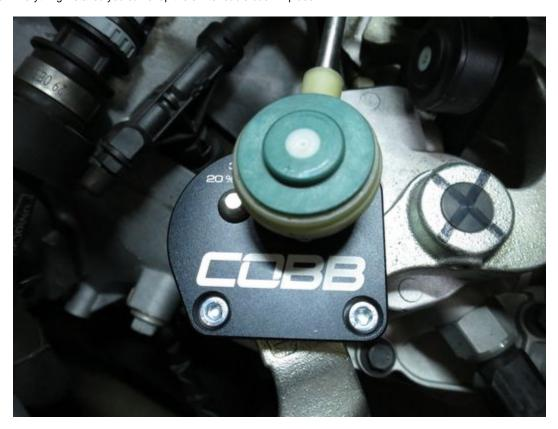
14. It's usually a good idea to now adjust the neutral position of the shifter, so with the shifter in Neutral, release this white clip on the cable nearest the fender.
