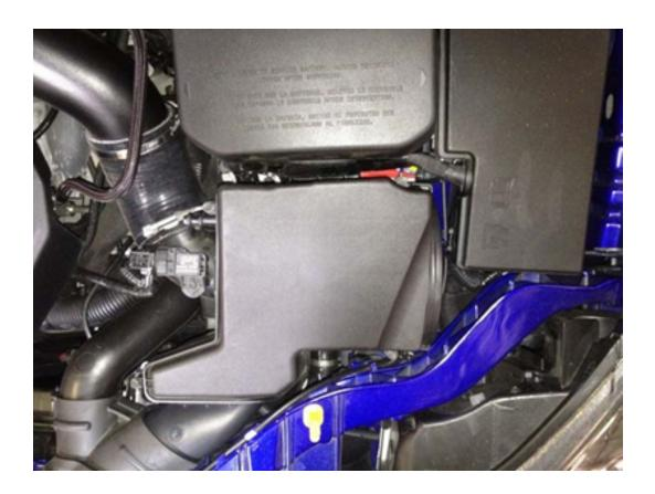
3. Using an 8mm socket, loosen the clamp that secures the airbox to the turbo inlet tube until there is slack. Socket size may vary depending on the intake that is installed.
